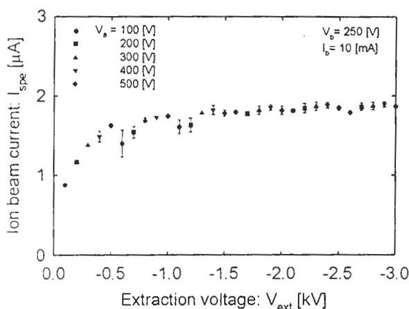
Figure 2. Ion beam current versus extraction voltage,  $V_{ext}$ , for acceleration voltages ranging from 100 to 500 V
