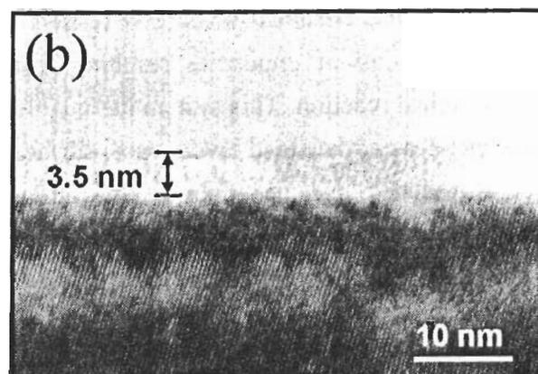
Figure 3. TEM images of (a) damaged layer on Si surface induced by  $Ga^+$  ions at 25 kV and (b) 200 eV  $Ar^+$  ions after 3 hours of finishing at an incident angle of 30 degrees
