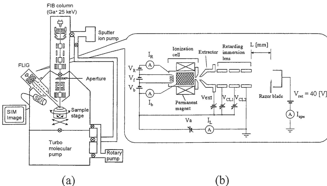
Figure 1. Schematics of (a) FIB-FLIG apparatus for TEM specimen fabrication and (b) developed compact FLIG
